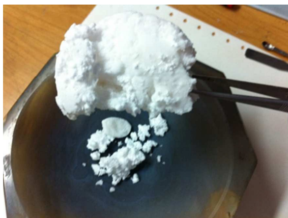
Fig. 3 Photograph of the glass electrolyte after synthesis
