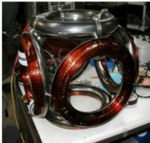
Coil winding inside Polywell device
