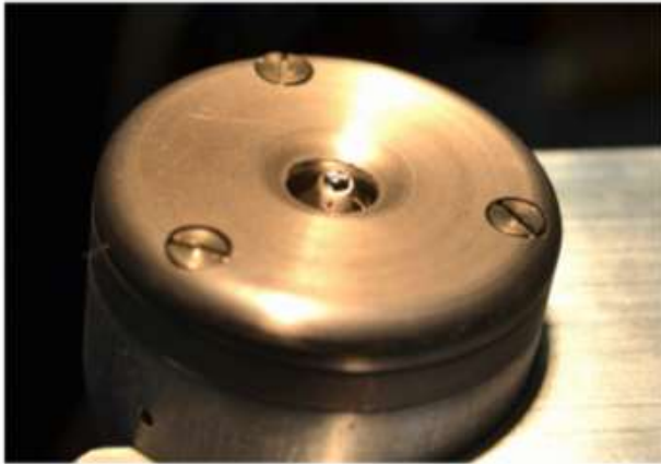
Solid arc with 2 mm gap using polypropylene film
