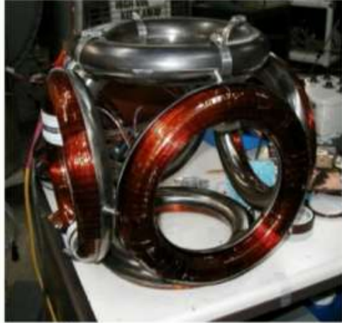
Coil winding inside Polywell device
