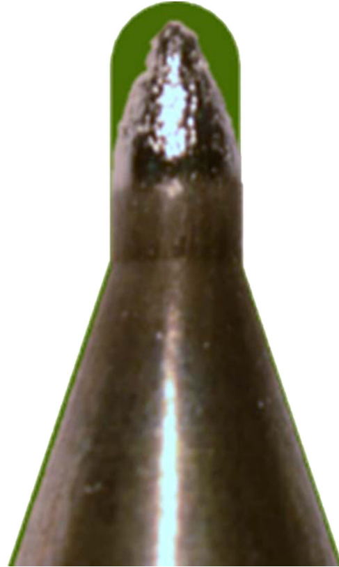
FIG. 7. A close-up photograph of a tungsten cathode after about 200 plasma injections. The width of the central tip is 2 mm and the green area highlights material erosion.
